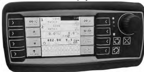
IntelliAg MVT Virtual Terminal 4" Display
