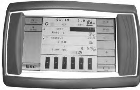
IntelliAg MVT Virtual Terminal 7" Display
