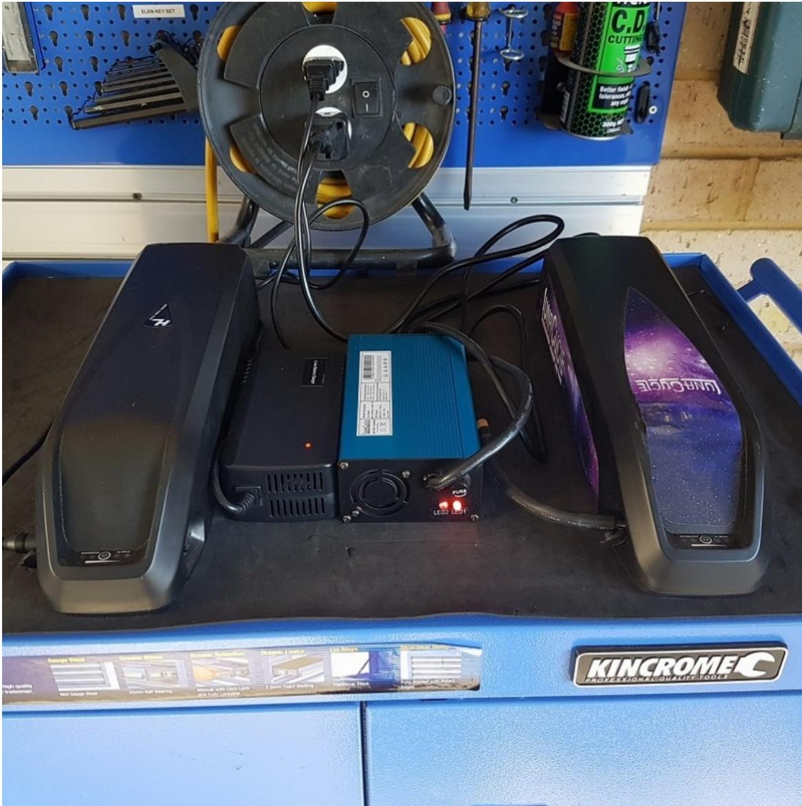
5. When the battery pack is fully charged the charger will stop automatically and the LED will turn **green**, and if you used the wrong charger or it's defective, the Battery Management System inside your Luna battery will disconnect the charger (Over 58.8V for a 52V, 54.6V for a 48V battery). But it's always good to double check if you have the good charger!
