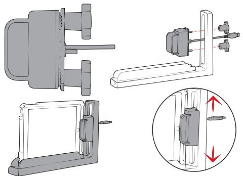
Remove thumb screws, position the GDS Slide Dock Module on the vertical slide rail and tighten the knobs.
