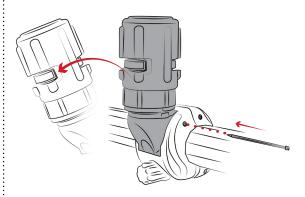
Once roll pin is removed the existing product can be removed to expose mounting slot.
