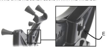
4. ONCE (E) SCREW IS THREADED BY HAND INTO (F) NUT, STRAIGHTEN (B) SUPPORT SLIDE AND FULLY TIGHTEN USING SCREWDRIVER
