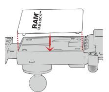
Secure using (J) screws on back of slide assembly. Lock must be engaged to access all four holes as shown.
