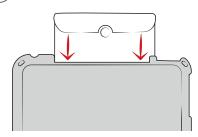
On the back of the top slide, review the numbers shown in the middle. Take note of the lowest number that is fully visible. This reference will help you in the next step. In this example, the lowest visible number is 8.
