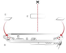
Carefully insert the device into the prepped Bottom Enclosure (B) ensuring positive connection with the USB connector. Then connect the Bottom Enclosure (B) to the Top Enclosure using the two Bolts (C) and sandwiching the rubber gaskets (D).
