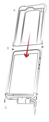
When using included RAM® Cable Clamp (G) be sure to attach the accompanying foam insert into the longer side of the bracket when using Type A USB cables for greater stabilization.
