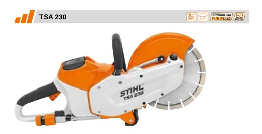
TSA 230 // Manoeuvrable battery cutoff machine for wet cutting indoors and out. 230 mm cutting wheels up to 70 mm, water connection with ball valve and hose coupling, spindle lock, maintenance-free belt drive.
