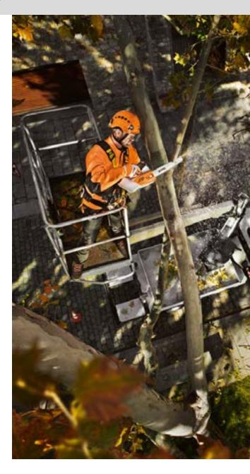
MSA 160 T // Very lightweight battery arborist saw for professional work in noise-sensitive areas. Captive nut on the sprocket cover, side chain tensioning, PM3 <sup>1</sup>/<sub>4</sub>" saw chain as standard for a clean cut and good cuttingperformance.
