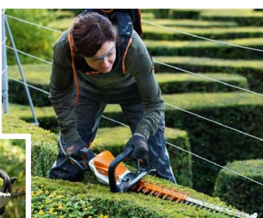
The rotating multi-function handle of the HSA 94 makes vertical cutting even more comfortable.
