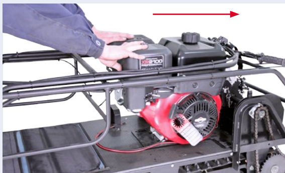
6 Move the engine bracket forward.
