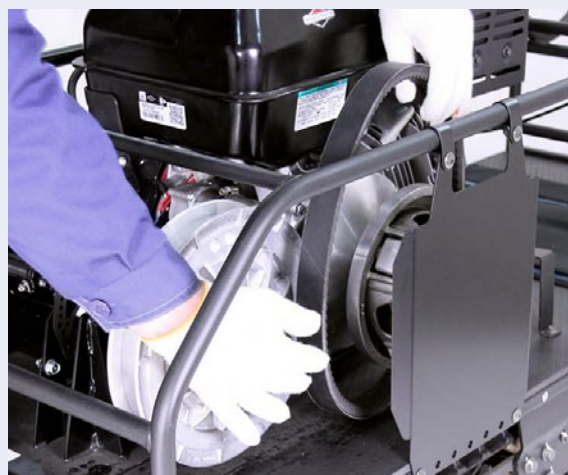
10 Remove the CVT belt.
