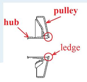
If there is ledge — the moving sheave can be blocked on the bushing.
