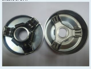
3.4. Align the rail and rollers and assemble movable sheave.
