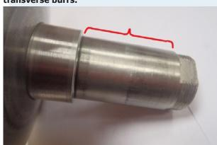
2.5. Check the inner surface of the movable sheave CVT. Transverse burrs should not be.
