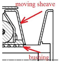
If there is ledge on a pulley, it is necessary to grind off it.
