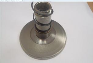
3.6. Hold assembled movable sheave and install it on the shaft CVT.
