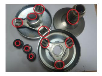
Use non-freezing lithium lubricant (for example, TEXACO STARPLEX EP 2) or aerosol lubricant for motorcycle chains.
