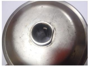
If the CVT is assembled correctly — you can see a bronze bushing.
