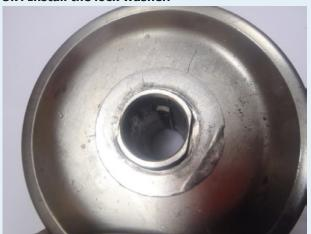
3.8. Install and tighten the nut. Fold lock washer for fixing nut.
