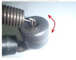
If the rollers rotate bad — check clips.
