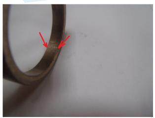
Sharp edges must be grind off and sanded.
