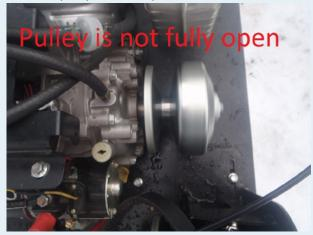
To resolve this problem it is necessary to disassemble the drive pulley and check all its parts. Then upgrade the CVT and lubricate it.
