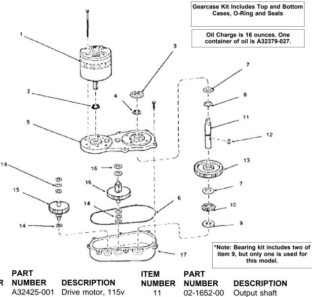
NUMBER 1 2 Oil seal 02-2853-01 12 03-1364-00 Woodruff key 3 Water shed 13-0709-02 13 02-1653-00 Output gear 4 02-1607-00 Oil seal 14 Washer 03-1408-24 5 A31230-001 Gear case kit First gear & 2nd pinion 15 02-2072-00 (cover and case) 2nd gear and 3rd pinion 16 02-2071-00 6 A26103-001 O-ring 17 A31230-001 Gear case kit 7 02-1681-00 Thrust race 18 03-1252-01 Screw 8 03-1393-01 Retaining ring 19 A32402-021 Complete gear and 9 02-1679-00 Thrust race motor assembly 10 A32368-020 Bearing kit\*
