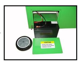
connected to the red terminal and black wire to the black terminal. Care must be taken to ensure you put the battery terminals to the top left side when you insert the battery into the cage.
