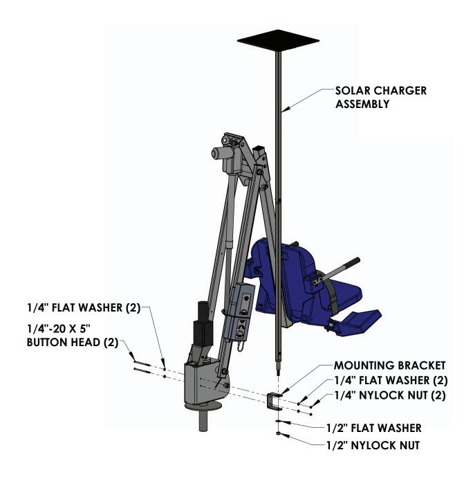
Begin by installing the solar charger assembly to the mounting bracket with the 1/2" flat washer and nylock nut using a 3/4" wrench. Next, intall the mounting bracket to the lift with 1/4" x 5" button heads, 1/4" flat washers and 1/4" nylock nuts using a 1/8" allen wrench and 7/16" wrench.
