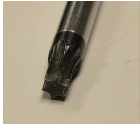
"TORX" T20 DRIVER FOR OPENING CONTROL-BOX
