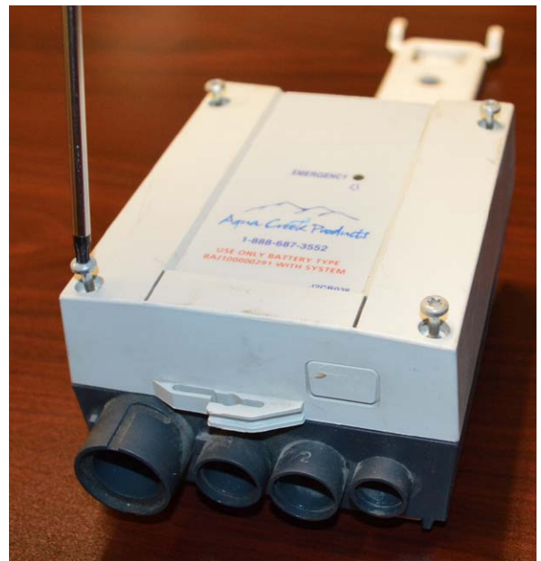
REMOVE THE FOUR (4) SCREWS FROM THE TOP OF THE CONTROL BOX: LEAVE SCREWS IN HOLES
