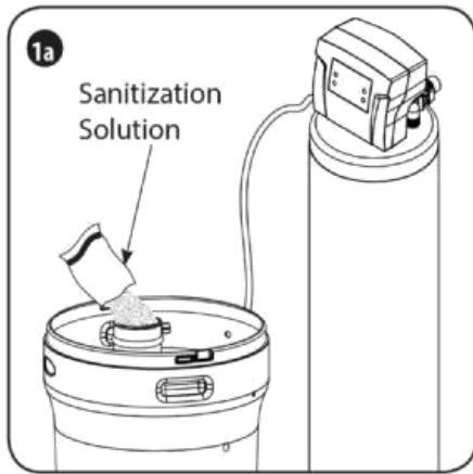
1a. Pour entire packet of Sani-System Liquid Concentrate – Part # 50032 (24 packets) into the brine well. If no brine well is present, pour entire packet into bottom of brine tank when salt is nearly empty.
