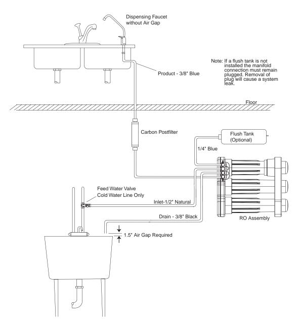
Figure 2 Typical Basement Installation
