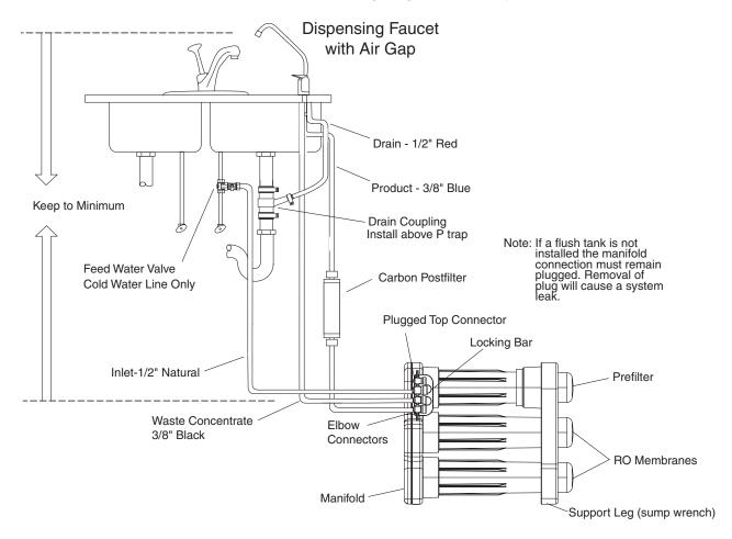
Figure 1 Typical Under-Sink Installation
