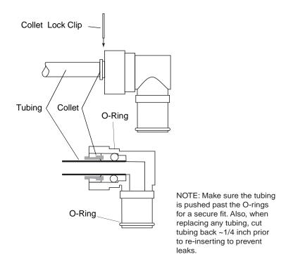
Figure 4 Side View and Cutaway of Tubing Fitting
