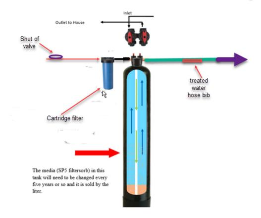
**b)** Verify that the water softener valve is in the bypass position.
