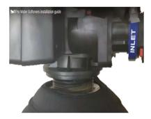
8) Install the bypass valve to the control valve.
