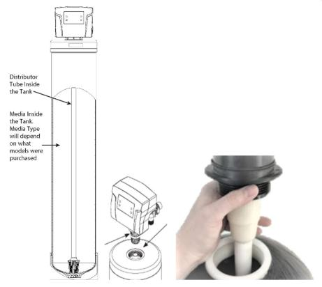
Carefully screw the control valve onto the mineral tank. Hand tighten ONLY. (The "O" ring of the control valve will seal the tank.)
