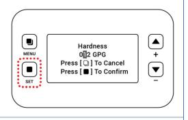
4. Use **UP** and **DOWN** arrows to select the appropriate hardness (GPG) levels.
