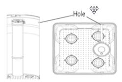
c) Insert the brine well with float into the large hole on the grid plate (round or rectangle).
