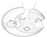
i. Align the brine well cylinder to the small brine line hole near the top of the brine tank. (This is where the brine line will slip through.)
