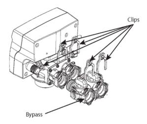
g) Press the bypass valve into the SoftPro control valve
