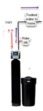
**b)** Verify that the water softener valve is in the bypass position.
