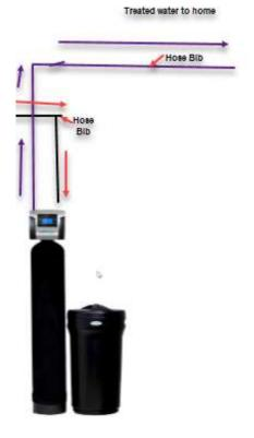
**b)** Verify that the water softener valve is in the bypass position.
