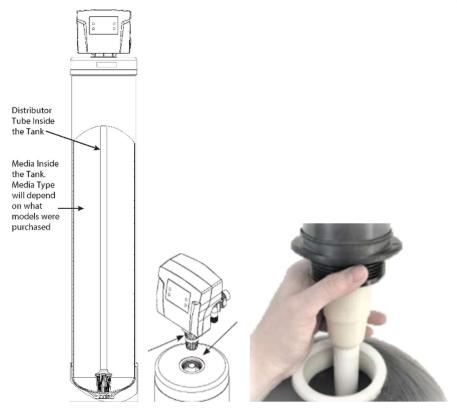
c) Carefully screw the control valve onto the mineral tank. Hand tighten ONLY. (The "O" ring of the control valve will seal the tank.)
