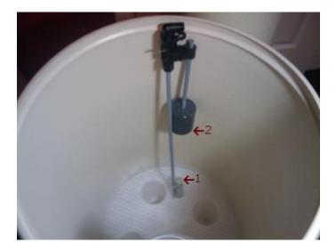
$\Box$ Slide the float assembly into the brine well shown in photo below and stick the stud into the side hole on the brine well shown in photo below and secure it with the nut we supplied you.
