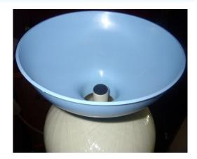
After adding the resin, remove the temporary cap, clean the valve threads with water, and screw the valve on. When screwing the valve on the tank the tube will slip into the bottom of the valve hole. Note no silicone or tape is NOT needed, the valve is o'ring fit and only needs to be tightened by hand.
