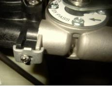
Remove the bypass valve shown in photo from the meter assembly by pulling it away from the meter assembly.
