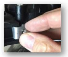
2. Position metal clips to clamp over the connection point and fasten with screw. Because the connection is O-ring sealed, it's important not to overtighten the screw. Overtightening will cause damage to the plastic assembly.
