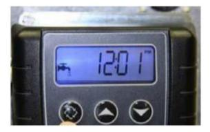
To enter master programming mode, press the UP and DOWN buttons together and hold for 5 seconds, and then release the buttons, as shown in picture below.
