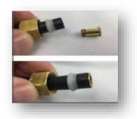
1. Prep brine line prior to install using brass nut, plastic Ferrule & brass tube insert.
