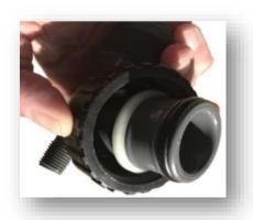
Assembling the two male pair 1" male treaded elbow adapters. You will be placing the nut followed by the white slip ring. Push the white slip ring down to the inner most groove. Next, slide the split ring onto elbow, placing in last groove. Repeat for remaining elbow.
