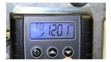
Once the time display is set to 12:01 PM, press the "extra cycle button once as shown in the photo below.
