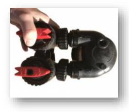
1. Lube O-rings on the bypass valve and attach bypass valve to the in/out head, fitting the female ends with the easy tighten nuts onto the female ends of the in/out head. Hand tighten the nuts to seal the connection between the bypass valve and the in/out head.
