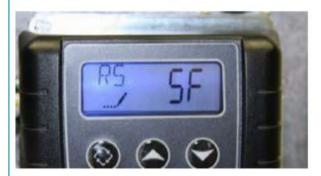
The display should now show SF 10 as shown in the picture below. This indicates the Safety Factor is 10 percent. Use the UP or DOWN button to change this value to 15. Press the Extra Cycle Button once.
