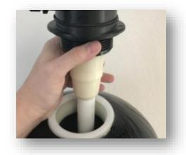
3. Verify that the basket is securely fastened to the in/out head and connect with distributor tube located in the carbon tank. Make sure that the tube is inserted into the basket. To secure in place twist clockwise till tight
