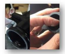
1. Apply silicone lube to the 2 'o'-rings on the valve and make connection. We also recommend applying silicone to the inside of the female end on the bypass valve.
