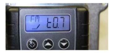
The system will now exit the Master Programming mode, and the display should now show the time of day, followed by the new number of gallons remaining, as shown in the picture below. Change the time of day by pressing and holding the UP or DOWN button until the proper time setting is shown. There is a PM light indicator to show the difference between AM and PM times.
