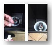
Locate predrilled hole in brine tank. Fasten brine well to side wall of brine tank using the white overflow elbow & plastic nut.
