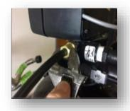
2. Connect provided brass nut to the Fleck valve. Be careful not to overtighten. Overtightening will cause damage.
