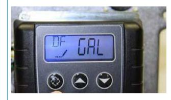
The display should now show VT St1b or df1b as shown in the picture below. This indicates Valve Type 5600 Mode) Do not change this value, and press the Extra Cycle Button once to continue.
