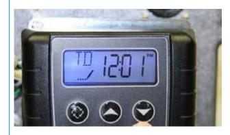
Once the time display is set to 12:01 PM, press the "extra cycle button once as shown in the photo below.
