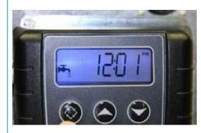
To enter master programming mode, press the UP and DOWN buttons together and hold for 5 seconds, and then release the buttons, as shown in picture below.
