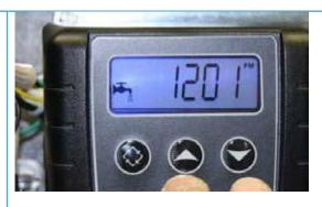
The display should now show DF GAL as shown in the picture below. This indicates United States gallons. Do not change this value, and press the Extra Cycle Button once to continue.
