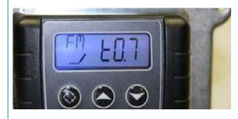
The system will now exit the Master Programming mode, and the display should now show the time of day, followed by the new number of gallons remaining, as shown in the picture below. Change the time of day by pressing and holding the UP or DOWN button until the proper time setting is shown. There is a PM light indicator to show the difference between AM and PM times.
