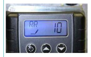
The display may now show BF 12 as shown in picture below. This indicates the length of the Brine Refill Cycle during regeneration. Change this value to the proper number for your system capacity below, and press the Extra Cycle Button once to continue. If this value is different, use the UP or DOWN buttons to change it.
