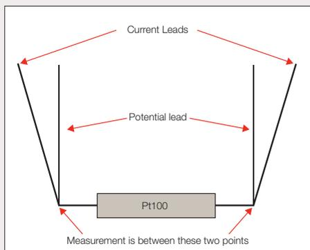
Two-wire sensors will also have large errors due to lead and connection resistance adding to the measured resistance value.
