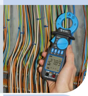
MD 9272 is a unique earth leakage clamp meter. It not just has the ability to accurately read the TRMS AC leakage current of a system, it can also detect losses in the system and suggest possible reasons for the loss. The voltage (AC/DC), frequency, power, harmonic, power factor (PF), total harmonic distortion (THD) and crest factor measurements make this instrument suitable for any electrician and engineer.
