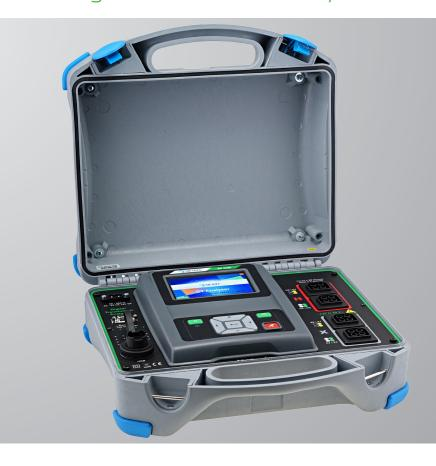
Digital Transformer Analyser (MI 3280) is a Multi-function, portable battery (Li-ion) powered test instrument with excellent IP protection: IP65 (case closed), IP54 (case open), intended for diagnosing of: turn ratio, phase deviation and excitation current of single and three phase transformers and winding resistance of single and three phase transformers
