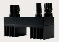
A four terminal resistance standard is constructed with 2 current terminals connected to the ends of the resistance element and 2 potential points connected at the adjusted value of the standard. This method of construction ensures repeatable values to be achieved when connecting to the standard's terminals.
