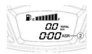
**ASR CALIBRATION PROCEDURE** In order to maintain the effectiveness of the ASR system following the replacement of one or both tires a calibration procedure of the system must be performed as follows on a straight flat stretch of road. After turning the ignition key to "ON" the ASR and ABS icons are flashing in same speed.
