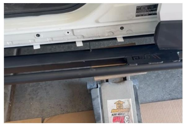
9. Slowly raise the floor jack and align the bolts with the opening holes. Use the retainer clips to help move the bolts around. (use caution when installing to not push the anchor bolts in. – otherwise you will need to use a magnet and lots of patience to remove the anchor bolt lost in the sill.
