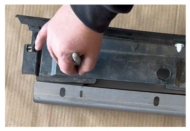
Install the anchor bolls into still section of the vehicle. Insert the long side through the hole first followed by short side. Rotate bolt to orientation shown below (3). Orientation of 3<sup>rd</sup> bolt from front is critical for correct side step fitment. (4)
