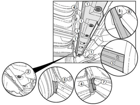
Remove the 8 x plugs (1) on the bottom of the still molding, 2 x clips (2) and 2 x screws (4) from the still moulding.
