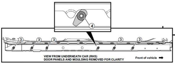
6. Pull down so mating surfaces of anchor plate and sill are flush
