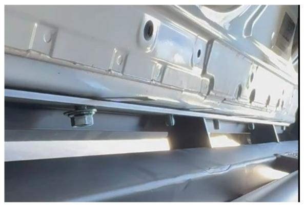
10. Once all the bolts are lined up, loosely install the M10 Flange nuts & washers.
