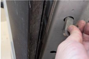
7. Install Bolt retainer clip on the threads of the anchor bolt near the top of the bolt with the end facing outwards of the vehicle. (This clip helps prevents the anchor bolt from being pushed in all the way.
