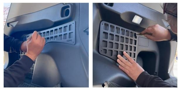
2. Drill a small pilot hole then use a 5/16" Drill bit to redrill the holes.
