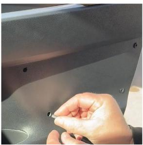
4. Install the ½" Aluminum spacers behind the molle panel and secure using the M4 Button head bolts.
