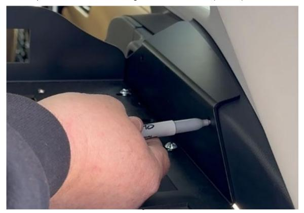
4. Remove the Cargo rack. Drill small pilot hole first then use a ½" drill bit.
