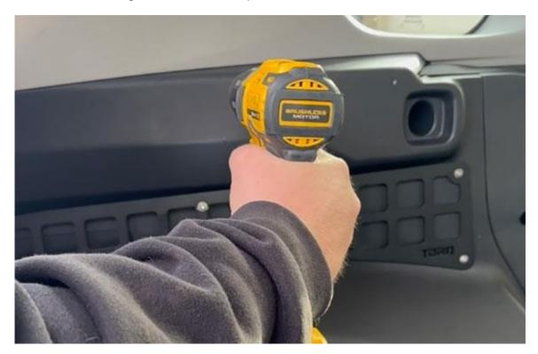
5. Install the 1/4" Rubber Well Nuts.
