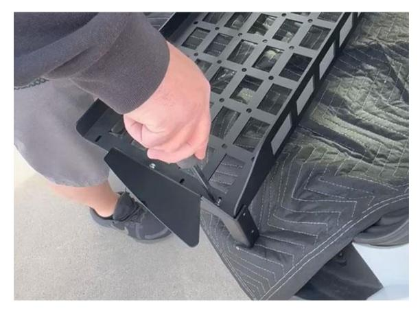
2. Test fit and align the cargo rack into the vehicle, Adjust as necessary.
