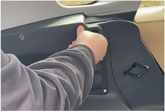
6. Reinstall the Cargo Rack and use the  $\frac{1}{4}$ -20 x 1-1/8" Button Head Screw to attach the cargo rack.
