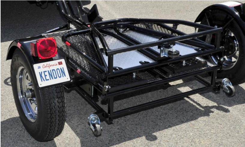
Trailer properly folded for transport when empty.
