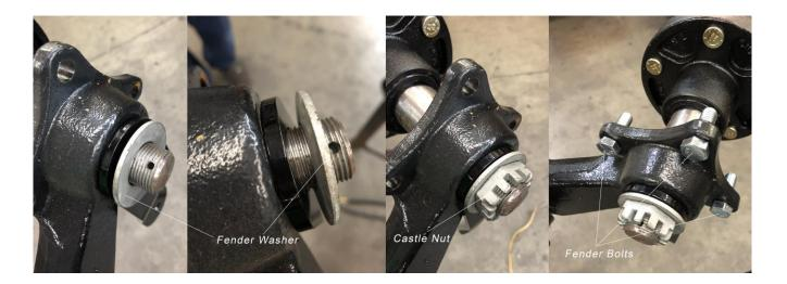
9. Attach the Fender to the Torsion Arm using Fender Bolts, Flat Washers, Lock Washers and Nuts and hand-tighten. Be sure the Fender Shell (top of the fender) or the top of the "Y" shaped fender bracket points towards the deck of the trailer. Note: The fender should be perpendicular to the deck of the trailer.
