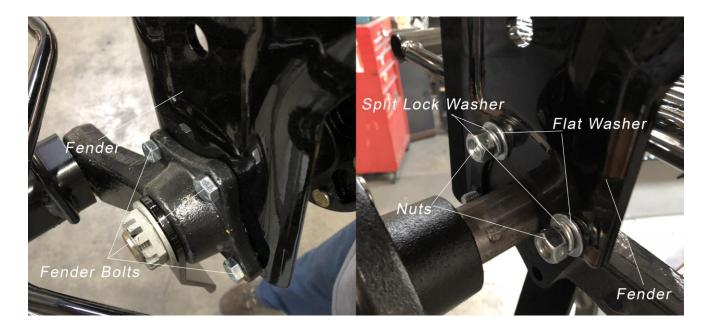
10. Rotate the Diagonal Bracket into its final position and attach using Bolt, Flat Washer, Flat Washer on opposite side, Split Lock Washer and Nut and hand-tighten.
