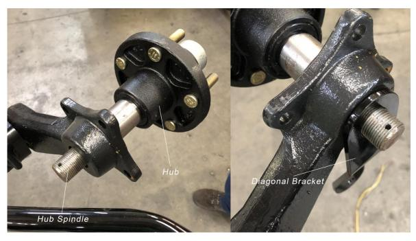
8. Attach the Fender Washer and Castle Nut onto the spindle and loosely hand-tighten. Be sure that the beveled edge of the Fender Washer faces the Torsion Arm and Diagonal Bracket. Insert the fender bolts through the torsion arm fender mounting holes. The fender is mounted using only three (3) of the four (4) mounting holes on the torsion arm. The topmost fender mounting bolt will be pointing towards the deck of the trailer, not the ground.
