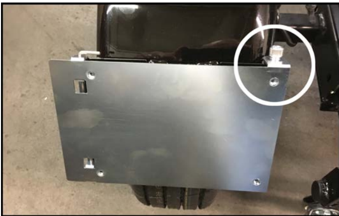
Photo: Tighten the thumbscrew on the closed SOLPH
