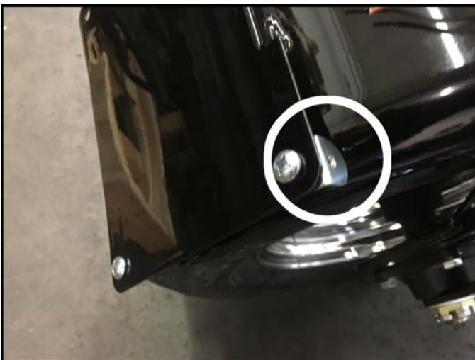
Photo: Small bracket installed properly
