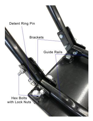
3. Attach the back of each left and right guide rail using the supplied hex bolts and washers using a 9/16" wrench.
