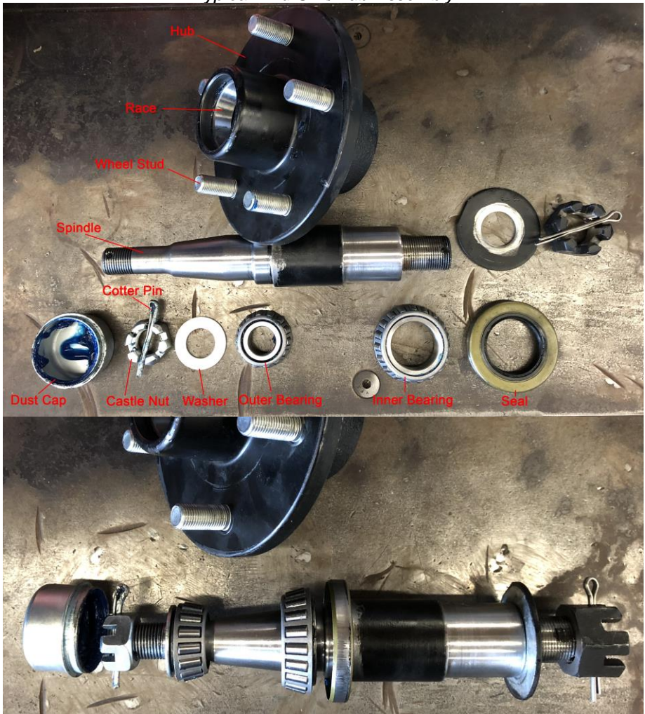
Typical End Unit/Hub Assembly
