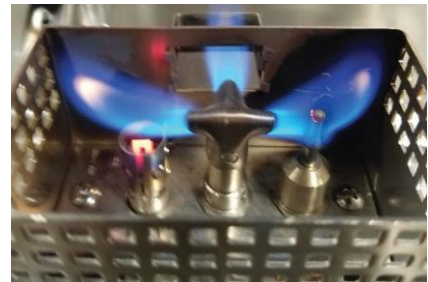
Figure 10.2 – Pilot flame coverage of thermocouple.
