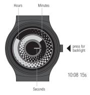
You can illuminate the display for a short time with the EL backlight by pressing the button. This function works best at night time.
