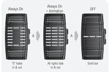
ALWAYS ON: The accelerometer is 'always on'. Shake your wrist (or press button A) to display the time.
