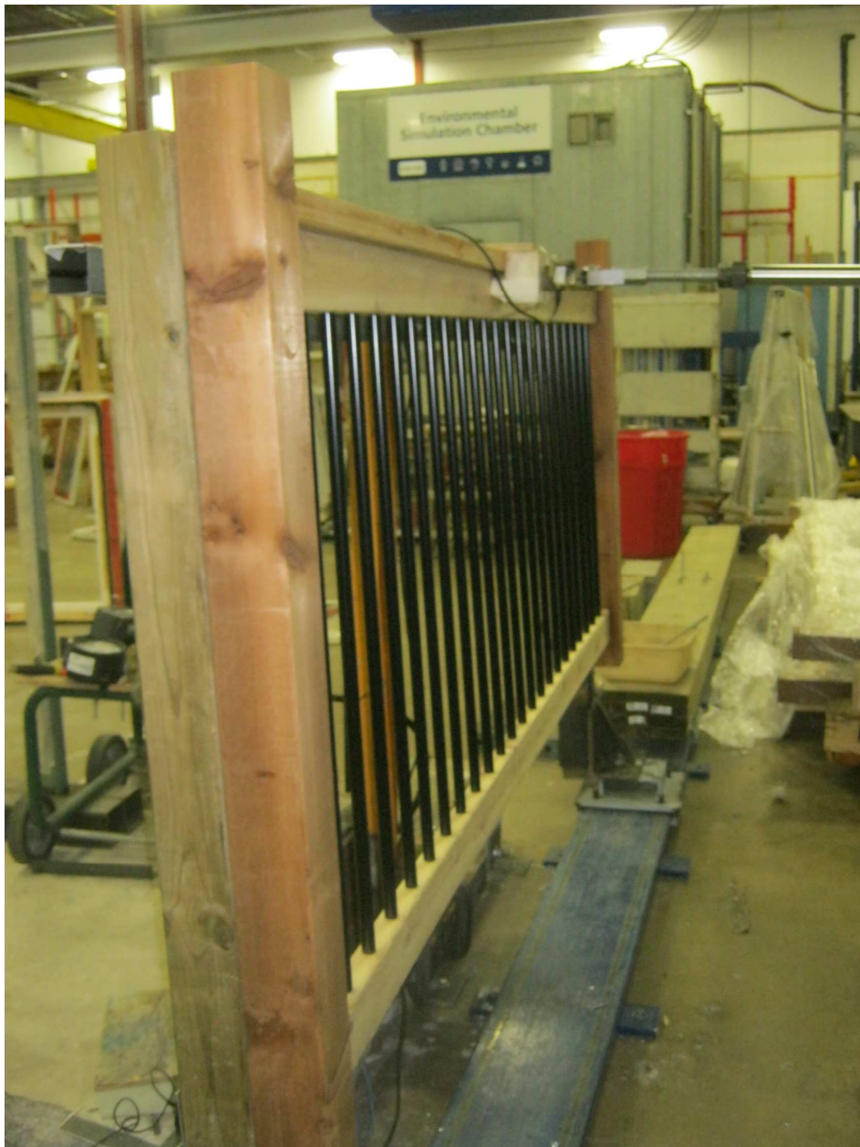
Photo 1 Guard with Polycarbonate Rail Connectors Undergoing Loading at Midspan
