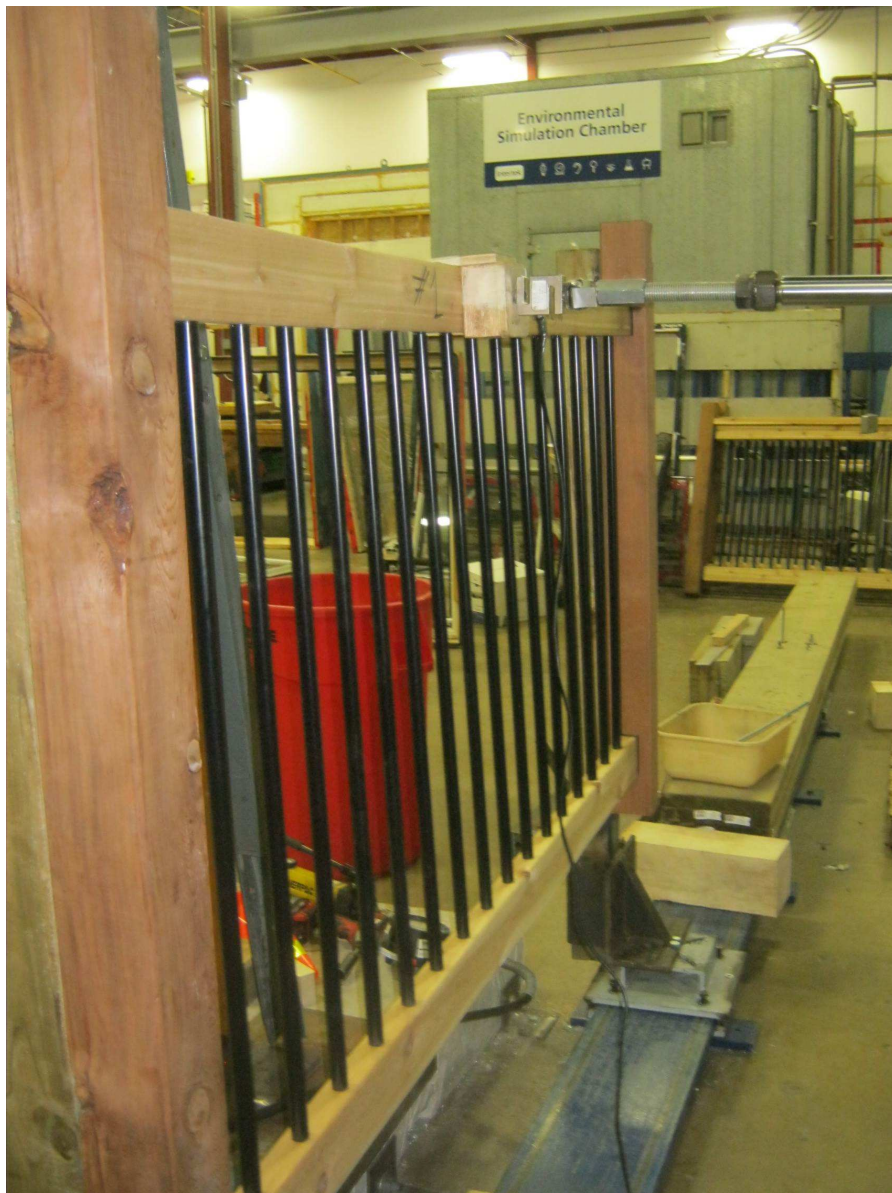
Photo 1 Top Rail Loaded at Midspan
