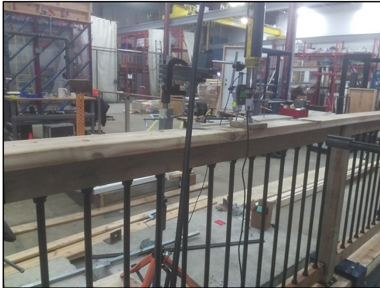
Photo No. 3 Vertical Top Rail Load Test
