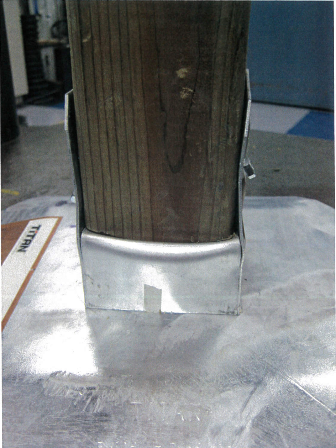
Photo 2 Post Bracket at Ultimate Load
