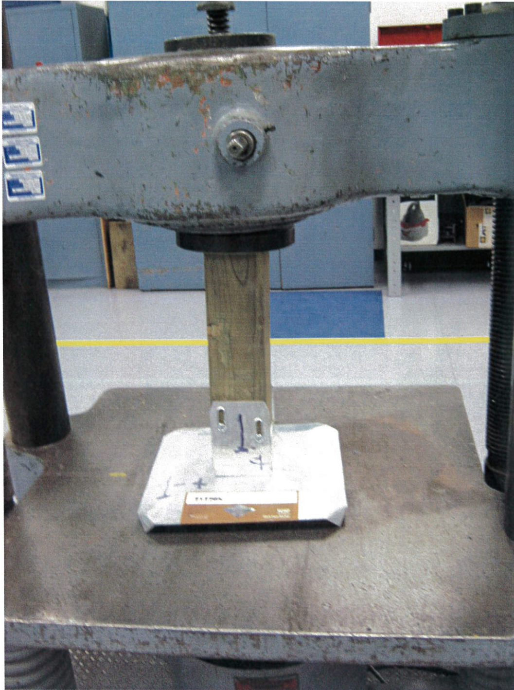
Photo 1 Deck Foot Anchor Set Up in Testing Machine
