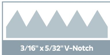
Trowel size is suggested to maximize coverage of membrane. Periodically check coverage during installation: 100% coverage is required. Uneven subflooring may require the use of either a leveling/patching material or a larger V-notched trowel for proper coverage.
