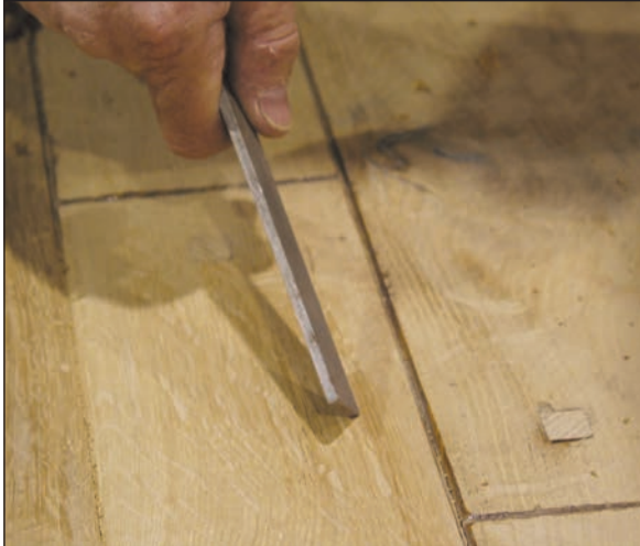
The side of a chisel creates dents.
