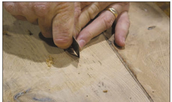
The edge of a putty knife creates larvae trails.
