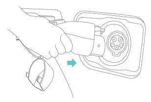
Note: The adapter must be plugged in within 1 minute of opening the charger door. Once it's plugged in, the adapter will automatically lock to prevent theft.
