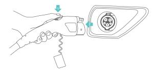
**NOTE:** The charger requires a 120 VAC split phase. It draws a maximum of 15 Amps of continuous current.
