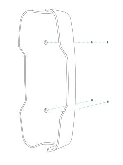
2. After inserting the wall anchors into the drilled holes, align and secure the mounting plate to the wall using the provided screws.
