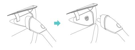
**Note:** Do not press the unlock button on the handle while pulling it out of the charge port.
