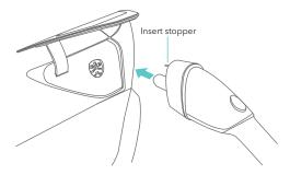
Note: The insert stopper on the adapter will keep it from being inserted too far and damaging the vehicle's charge port.
