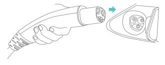
Charging begins automatically. Power will be delivered in accordance to the demand of your vehicle. While charging, the Charging Indicator will continuously blink. Always verify your vehicle-charging status by checking the vehicle panel.
